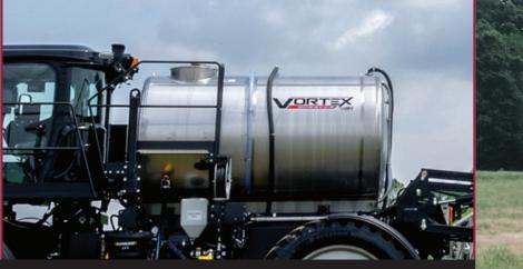
**COMBO READY** All units are equipped with an ISO hydraulic quick-connect bulkhead for a clean and seamless change from the liquid system to a dry spinner box.
