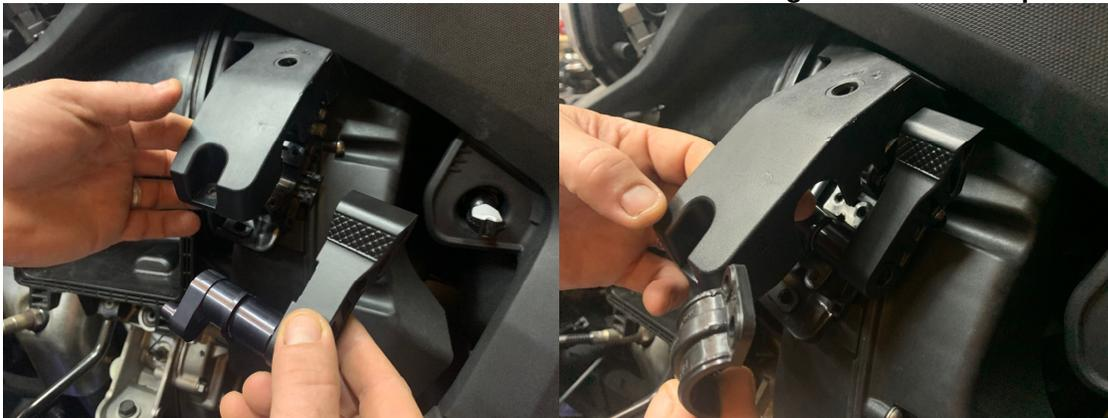
7.-Reattached the brake cable which may require you pull it downward to place over shaft.
