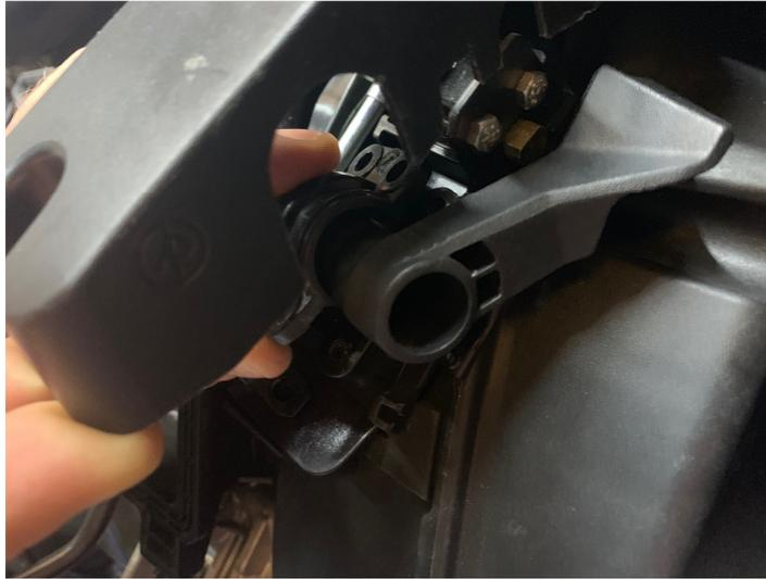
6.-Next install the new Brake Lever Assembly in reverse of how you disassembled the original. Then reinstall the shaft cover. Install the 4 bolts but do not tighten them at this point.
