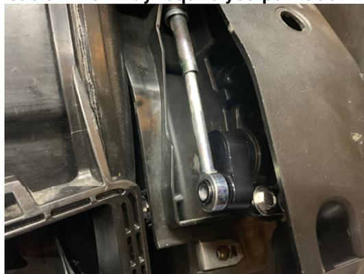
**8.-Once the cable is reconnected then tighten down all four bolts. Then lower the cover and reinstall the T-30 screw**
