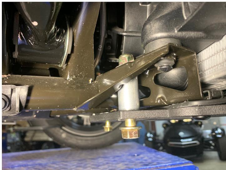
2.- Take the Supplied 3/8" bolts and place the supplied spacer as shown above. The spacer is located between the skid plate of the Grille Guard and the angled slotted gusset brace each side of the frame. Install the washer on top of the frame then the locknut.
