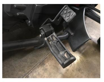
2.- Remove the frame support arm bolt.
