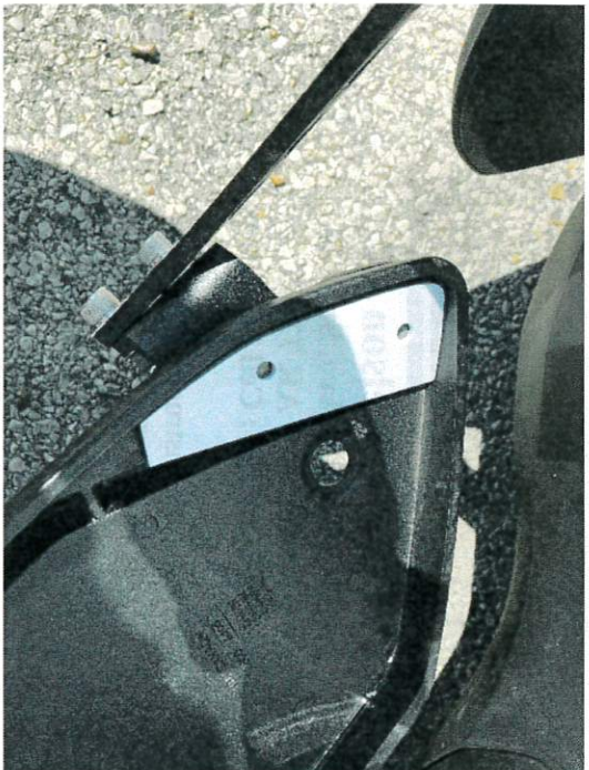
Left side install using drill template on Floor Board
