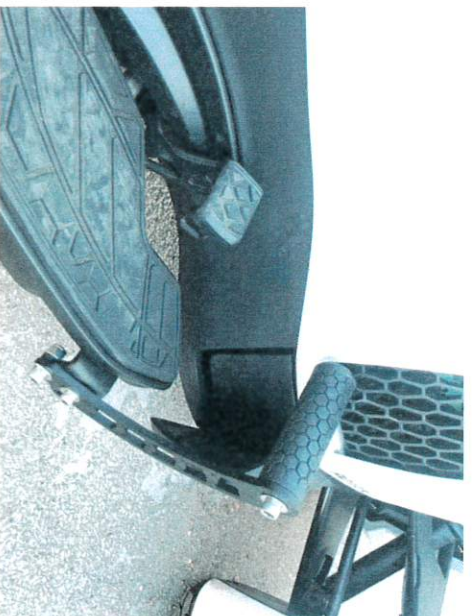
Right Side RT Road Peg Assembled on Floor Board
