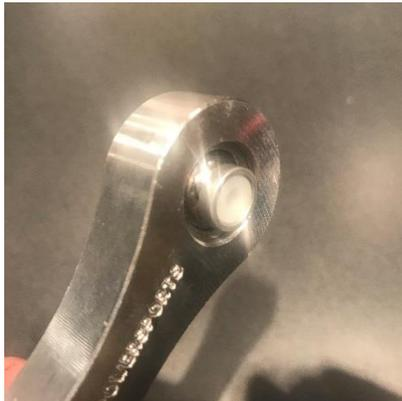
Take the install Nylon Insert and place it through the link top bearing. Place one spacer each side and you will see that the spacers once added fit flush with the nylon insert from side to side. This will hold
