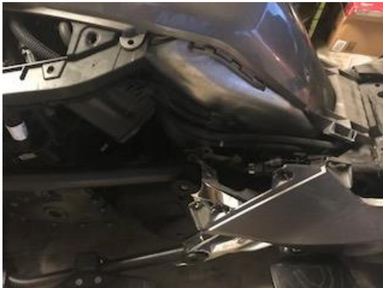
3.-Remove the lower left push pin connector then Lift up the lower panel which allows it to hang freely away from the frame.
