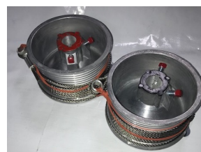
LEFT CABLE DRUM AND CABLE (RED) RIGHT CABLE DRUM AND CABLE (BLACK)
