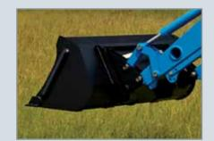
Quick attach, self leveling front end loader with skid steer compatible bucket (Optional) Easy to take off or attach loader and easily change loader attachments. With up to 3,065 lbs of lift capacity it outperforms others in its class. Grill guard comes standard with loader rather than an option like others in its class
